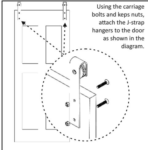
Using the carriage bolts and kept nuts, attach the J-strap hangers to the door as shown in the diagram.
