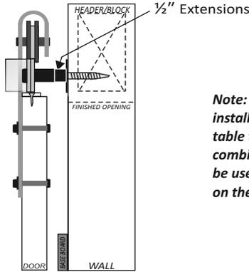
Standard hardware set + 1/2" or 1" extension kit installed where casing, base, or other trim is 1/2" thick or greater.
