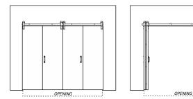
Doors will hang over into opening up to 4" on either side when in an open position [minimum 1" overlap on both sides]
