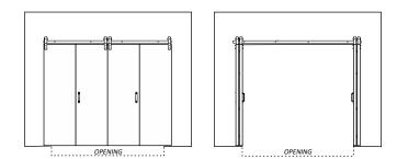
Doors will NOT hang over into opening, allowing for a completely **clear opening** *[minimum 5" overlap on stacking sides]*
