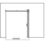
Door will hang over into opening up to 4" when in an open position [min. 1" overlap on both sides]
