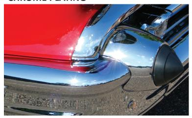
Chrome plating is an electroplating process in which a thin layer of chromium is applied to the surface of an object made from another kind of metal. Decorative car parts, for example, are often made from a steel base that is electroplated with a layer of copper, a second layer of nickel, and finally a third layer of chromium.
