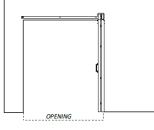
The stacked doors will hang over into the opening up to 4'' in the fully opened position, with a minimum wall overlap of 1'' on each side when fully closed.
