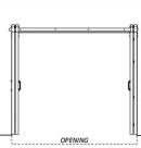
The stacked doors will hang over into the opening up to 4" in the fully opened position, with a minimum wall overlap of 1" on each side when fully closed.
