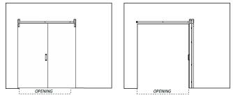
The stacked doors will not hang over into the opening in the fully opened position, with a minimum wall overlap of 5" on the stacking side and 1" on the closing side.
