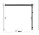
The stacked doors will hang over into the opening up to 4" in the fully opened position, with a minimum wall overlap of 1" on each side when fully closed.
