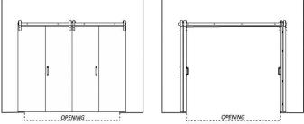
The stacked doors will not hang over into the opening in the fully opened position, with a minimum wall overlap of 5" on each side.
